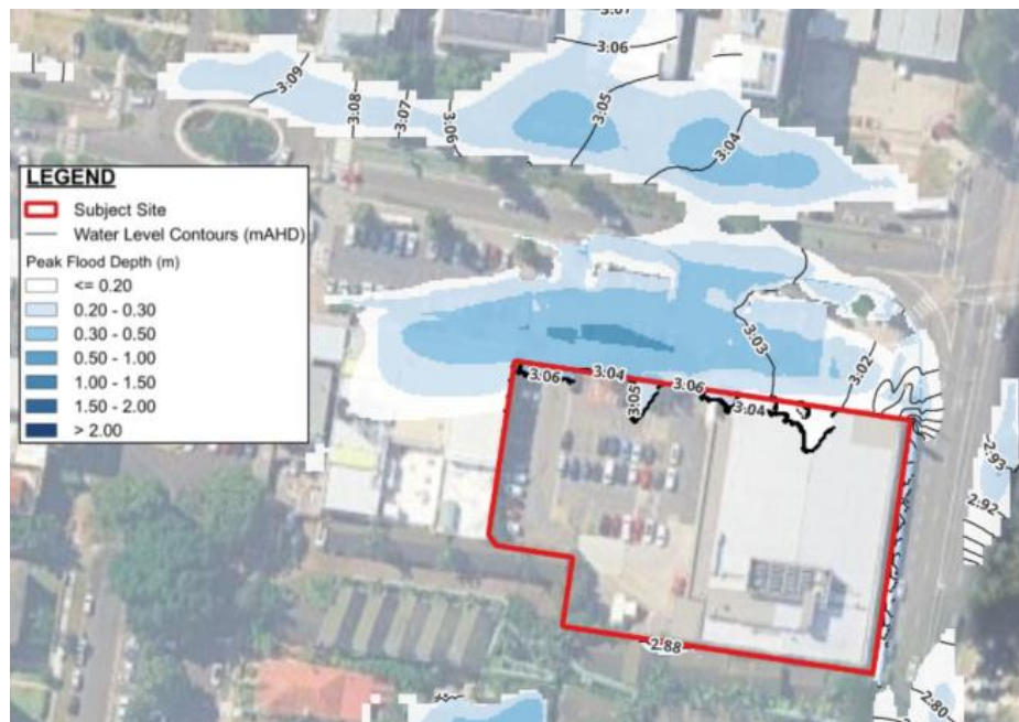
Figure 9: 1% AEP + Climate Change Event Flood Depths and Levels (Developed Scenario)
