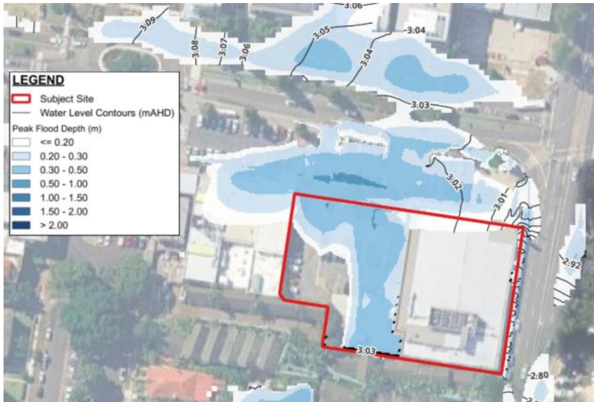
Figure 3: 1% AEP Event Flood Depths and Levels incorporating Climate Change (Existing Scenario)
