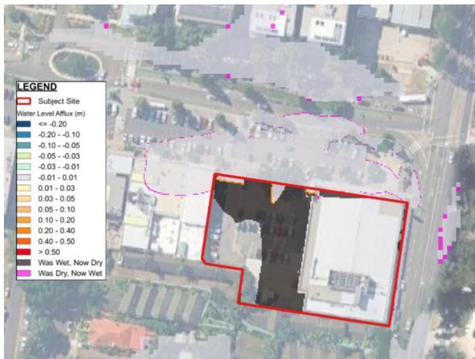
Figure 7: 1% AEP Event Flood Change in Flood Depth (Developed Scenario)
