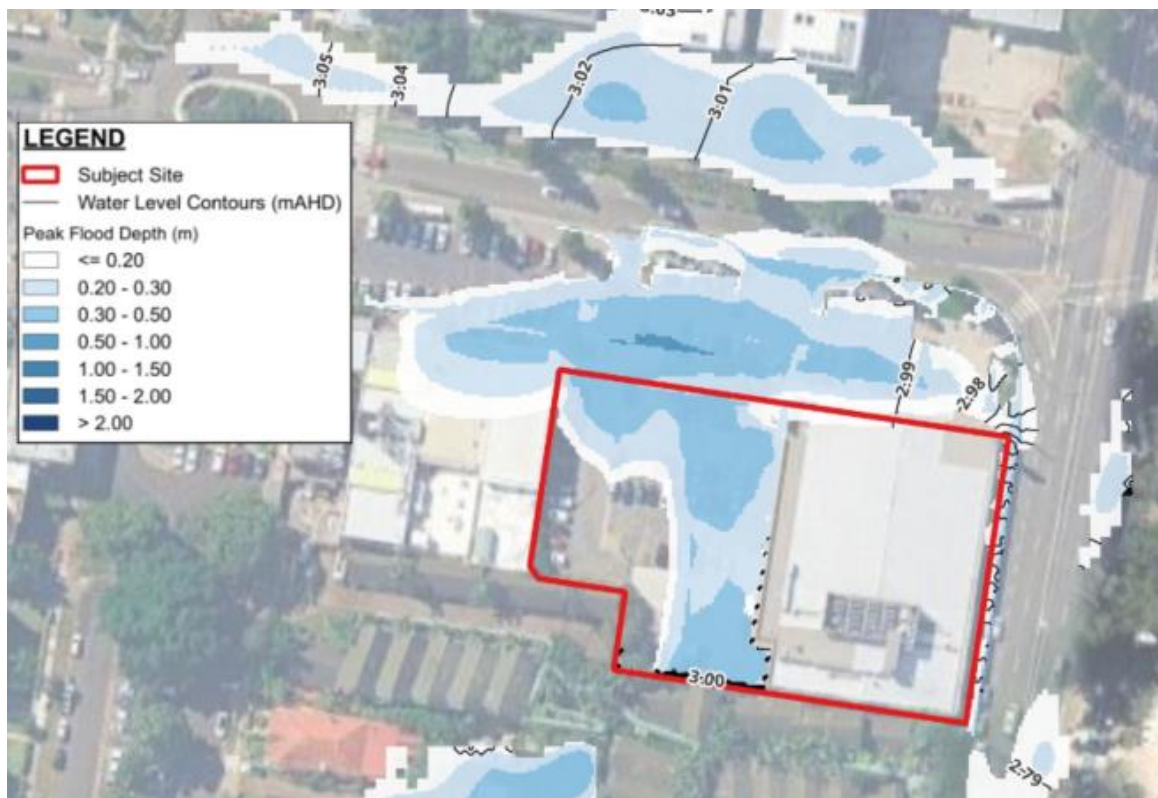
Figure 2: 1% AEP Event Flood Depths and Levels (Existing Scenario)
