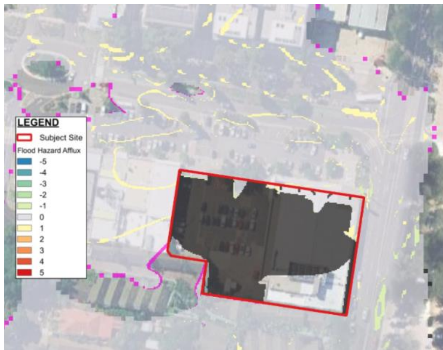
Figure 14: PMF Peak Hazard Afflux (Developed Scenario)
