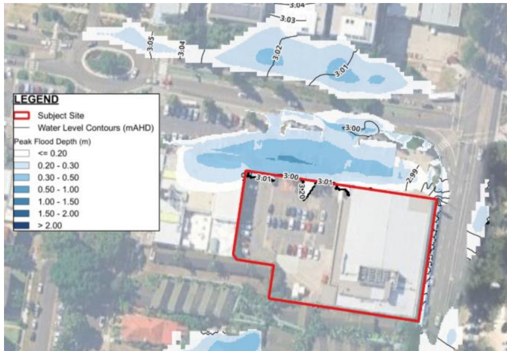
Figure 6: 1% AEP Event Flood Depths and Levels (Developed Scenario)
