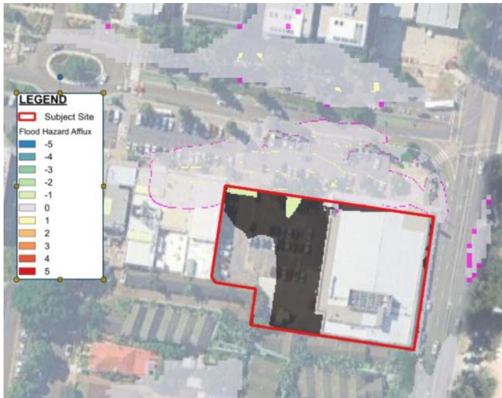
Figure 8: 1% AEP Event Peak Hazard Afflux (Developed Scenario)
