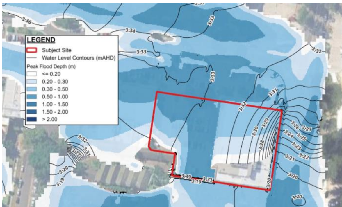
Figure 4: Probable Maximum Flood (PMF) Depths and Levels (Existing Scenario)
