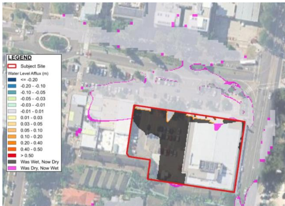
Figure 10: 1% AEP + Climate Change Event Flood Change in Flood Depth (Developed Scenario)
