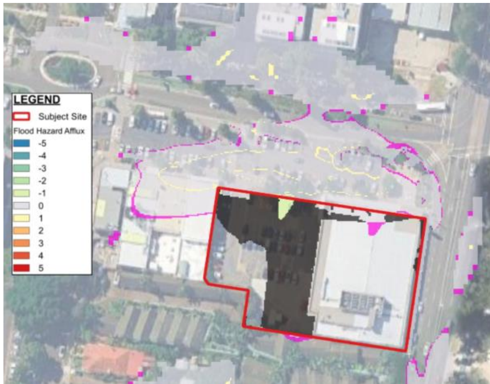
Figure 11: 1% AEP + Climate Change Peak Hazard Afflux (Developed Scenario)
